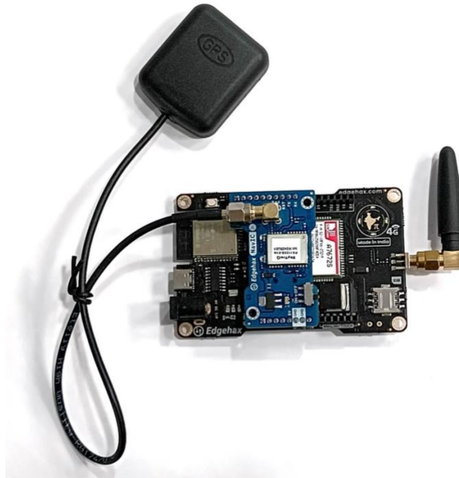
Edgehax NavIC Module Mounted on 4G module and connected to L1/L5 IRNSS Antenna
